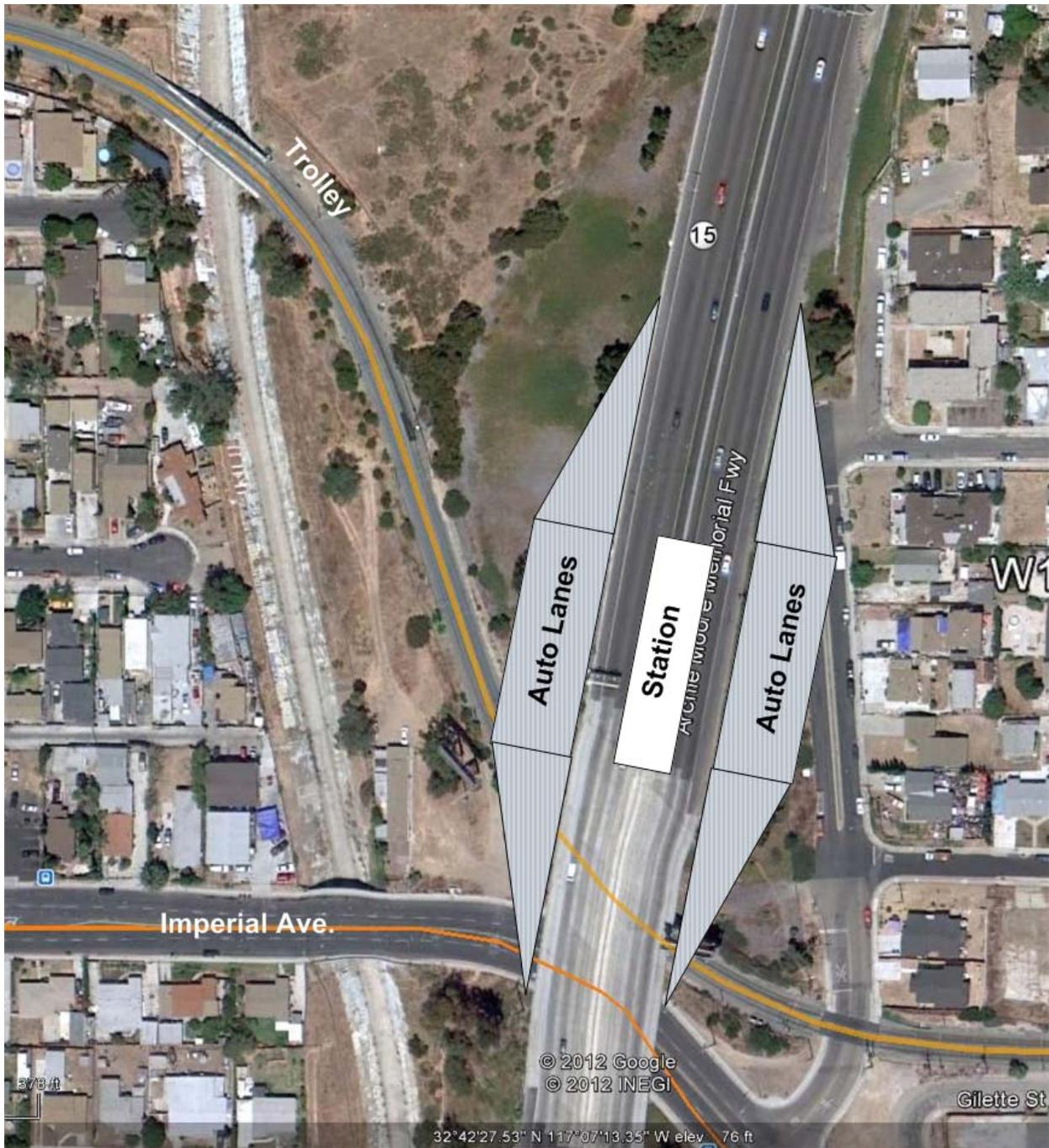
Figure 3, High resolution image showing the proposed moved auto lanes and station. The new trolley stop is located underneath the freeway bridge that crosses Imperial Ave. Access to the trolley stop(s) would be via Imperial Ave. Francis St. and/or Tompkins St.
